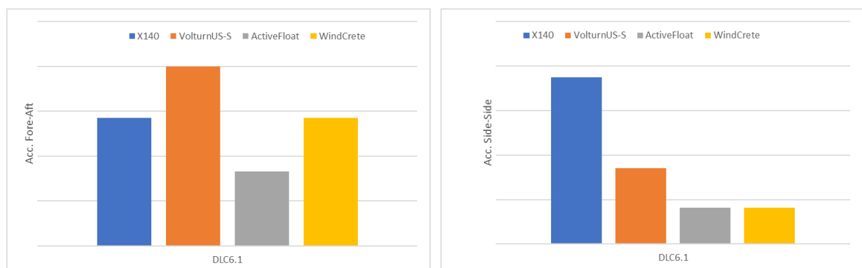
Figure 38 Comparison of the maximum accelerations in DLC6.1 for all the designs considered. Note that VolturnUS-S was evaluated for a typical US East Coast site, while the other concepts were evaluated for a Canary Island site.
